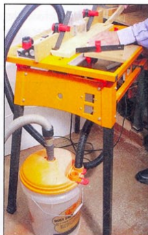
With a router table, both of the extract points can be linked to the collector
